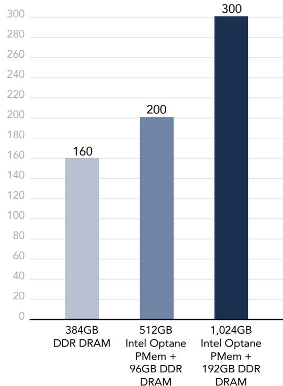
Figure 2: Number of VDI users on a four-server VMware vSAN cluster using View Planner. Higher is better. Source: Principled Technologies.
