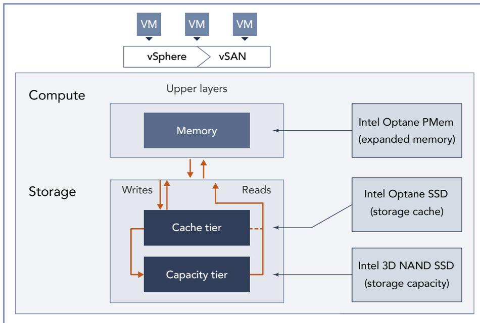
Figure 1: How Intel Optane storage and persistent memory work together
