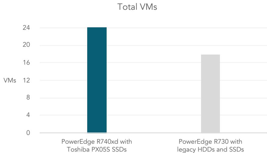
Our testing revealed that the legacy server configuration could only support 18 VMs, delivering 595,828 OPM. The Toshiba-Dell EMC solution demonstrated greater capacity, supporting 33 percent more VMs and processing 1,067,868 OPM—an 80 percent improvement over the legacy solution.
