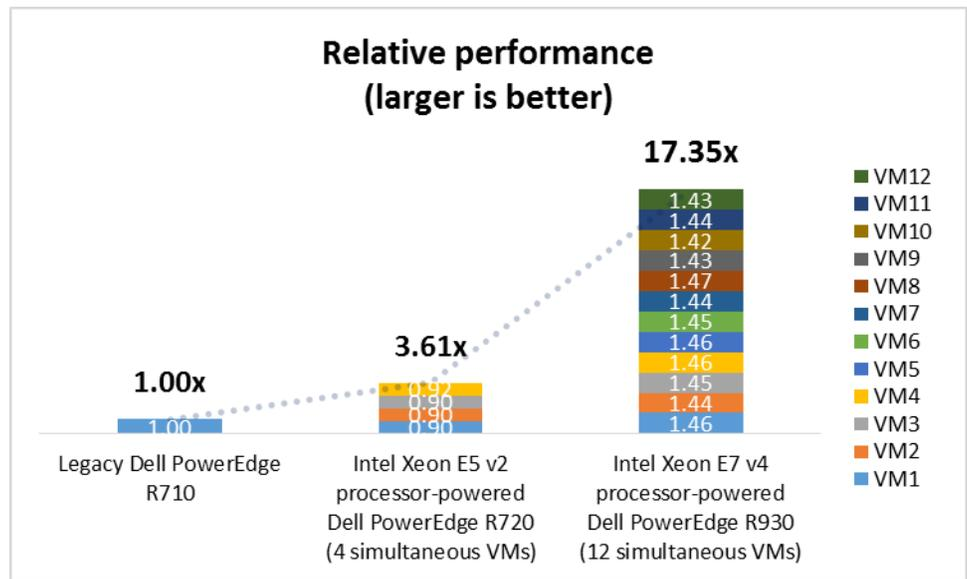
The VMs on four-socket server with Intel Xeon E7-8890 v4 processors completed the SAS workload in **30 percent less time**, on average, than the legacy server did.
