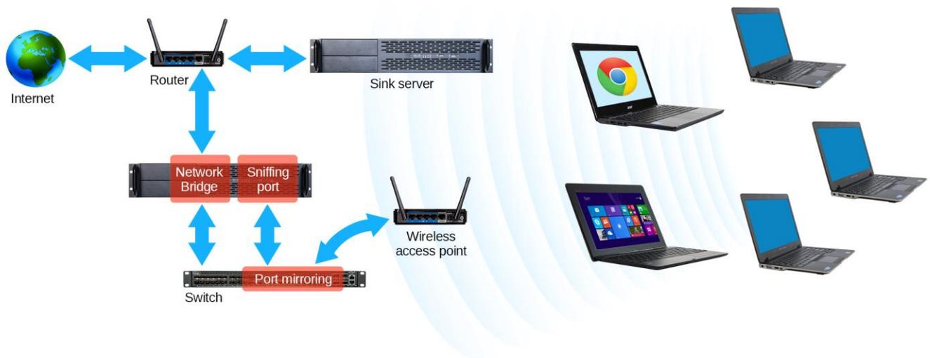
**Figure 8: Network configuration for packet sniffing.**
