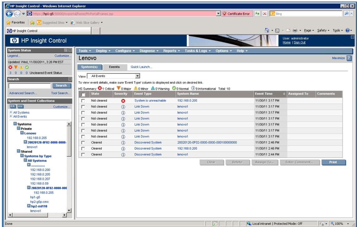
Figure 6. The Events tab showing that the network link is down.
