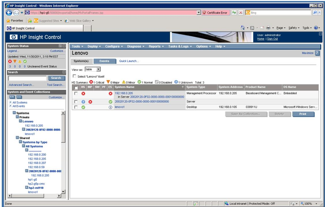
Figure 5. The Systems screen showing the loss of network connection.
