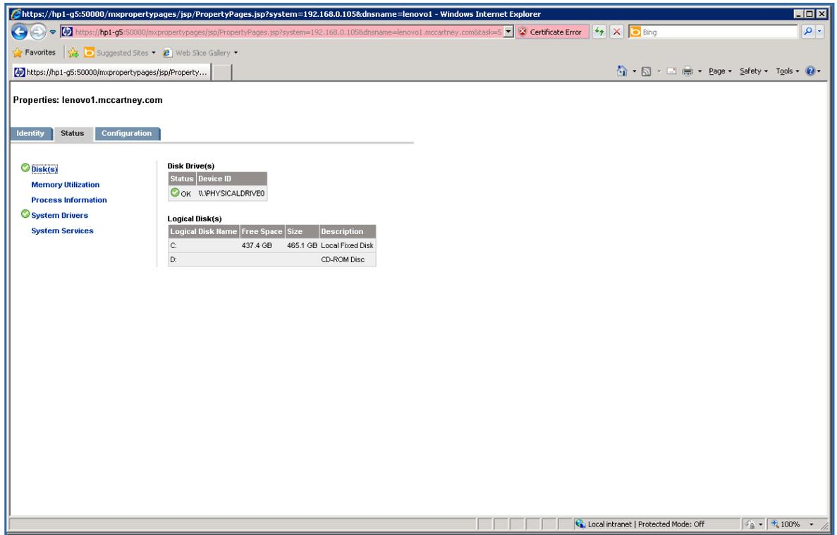
Figure 7. Disk Drive(s) Status screen based on WMI.
