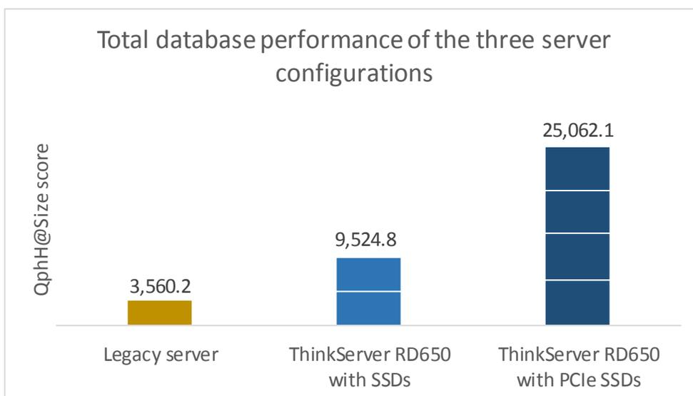
Figure 3 shows the average, per-instance database QphH@size score on each configuration, showing that not only was the RD650 able to support more instances, but that each instance was able to outperform the legacy server database instance.
