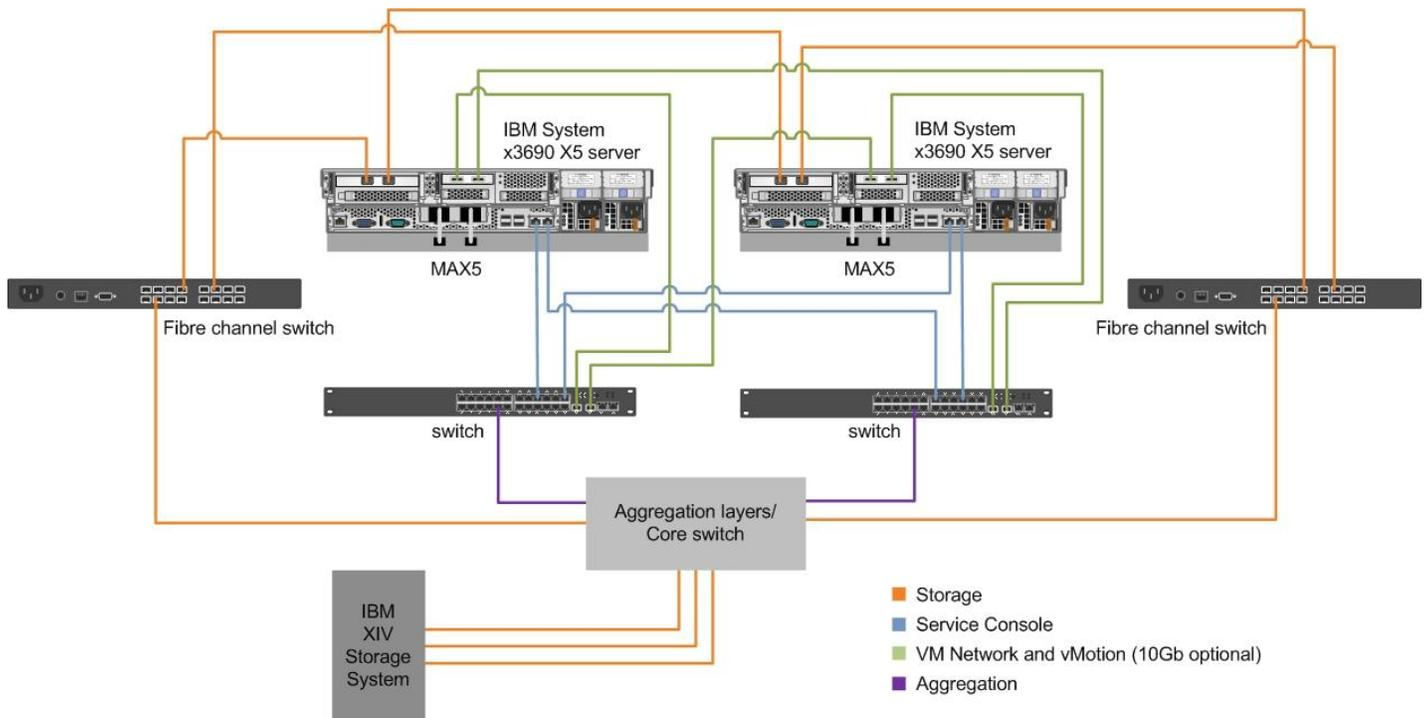
**Figure 22: Example diagram of network cabling.**
