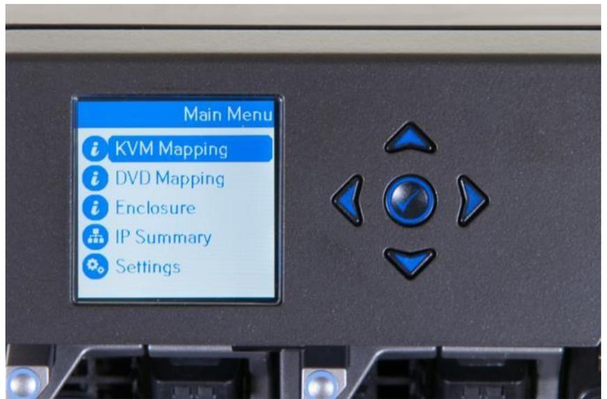
**Figure 1: View of the front LCD panel and arrow buttons.**
