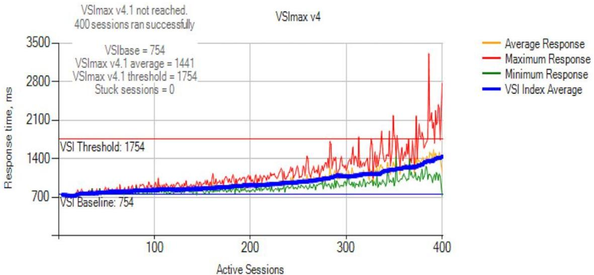
**Figure 7: The Dell PowerEdge FX2 using VMware Virtual SAN with four FC430 sleds ran 400 sessions (100 per server), with room to grow. VMware Virtual SAN 5.5 limits allowed only 100 sessions per server.**
