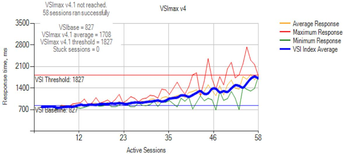
**Figure 6: The legacy Cisco server using a traditional SAN with a single B200 M2 blade ran 58 sessions and did not reach VSImax; Adding additional sessions caused the server to reach VSImax due to CPU saturation and unacceptable end-user response times.**
