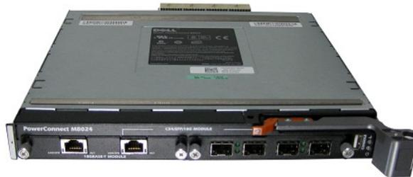
**Figure 1: The Dell PowerConnect M8024 switch.**
