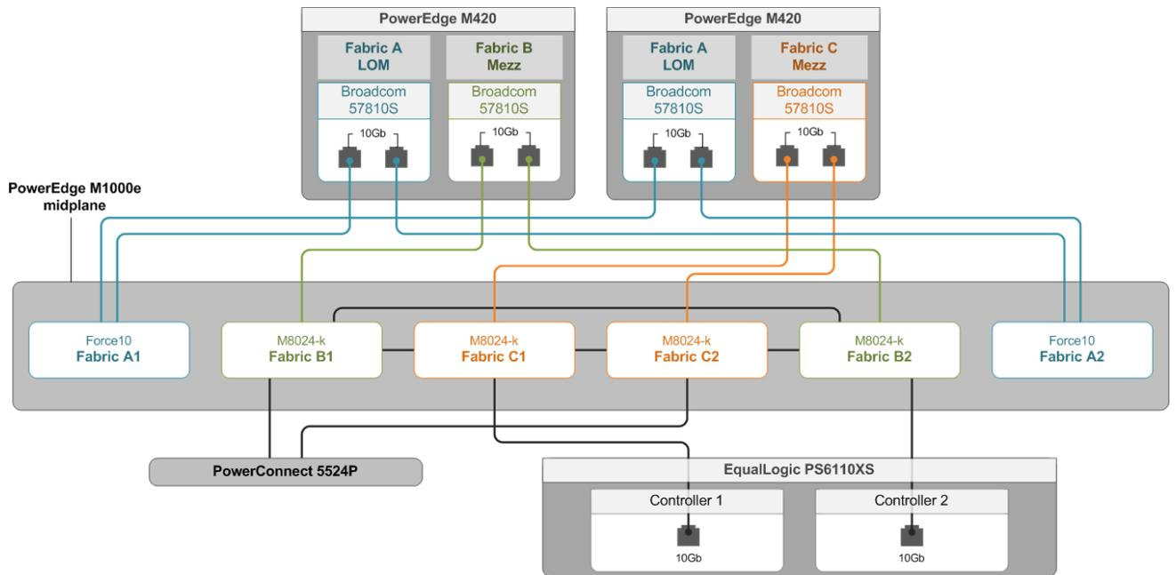
Figure 3: The topology we used for this reference architecture.
