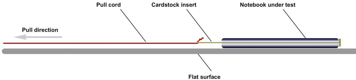
**Figure 8: Demonstration of method for pulling a netbook across a flat surface for the abrasion test.**
