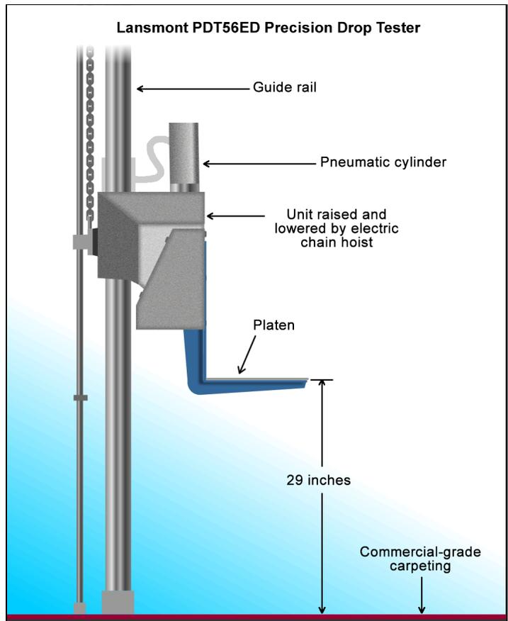
Figure 4: Our physical data protection test setup.
