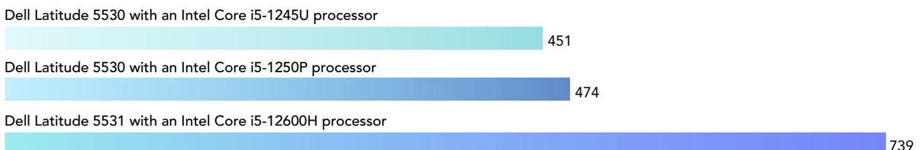
Figure 7: PugetBench for Adobe After Effects benchmark test results. We ran each test three times and report the median score. Higher is better. Source: Principled Technologies.
