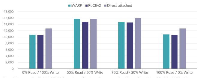
Figure 3: Average bandwidth (MB/s) for each read/write ratio we tested on the configuration with eight NVMe drives. Higher is better. Source: Principled Technologies
