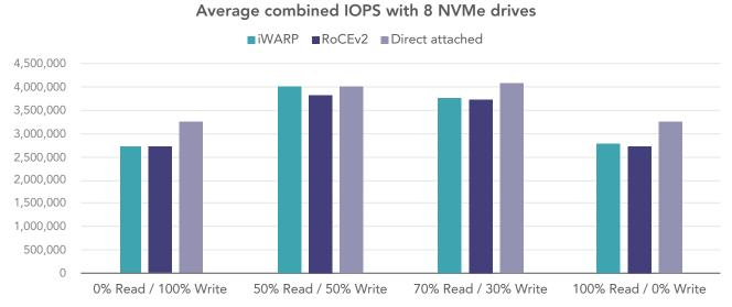
Figure 1: Combined IOPS for each read/write ratio we tested on the configuration with eight NVMe drives. Higher is better. Source: Principled Technologies
