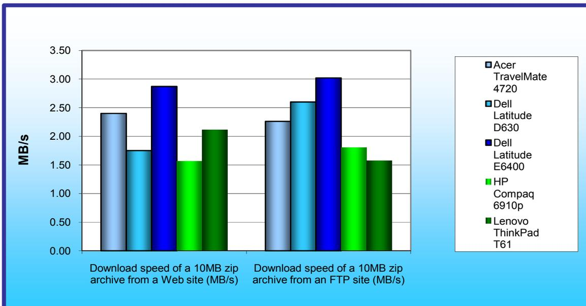
Figure 3: Download speeds in MB/s for the five test systems. Higher numbers are better.
