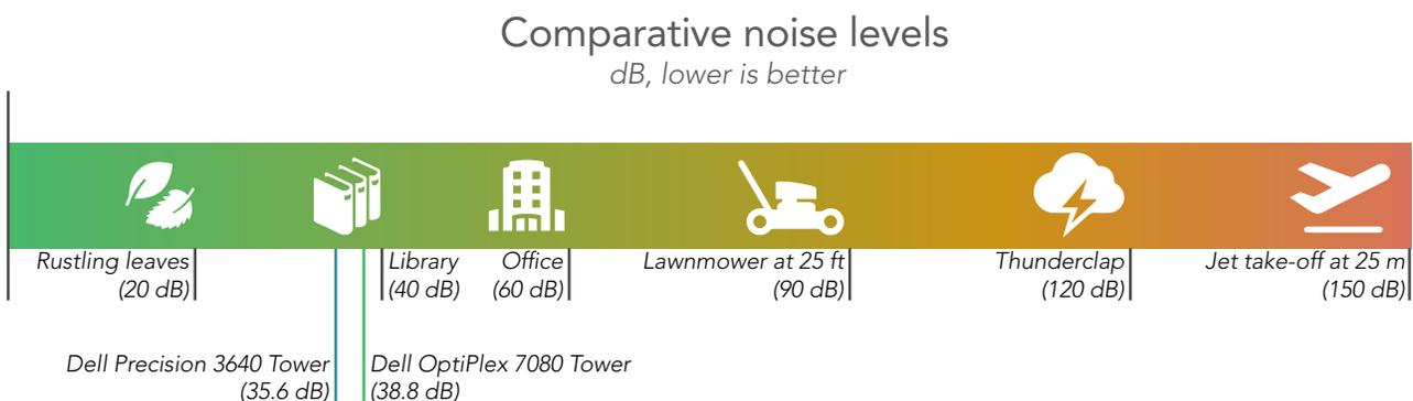
Figure 6: Comparative noise levels in dB. Lower is better. Source: Principled Technologies.
