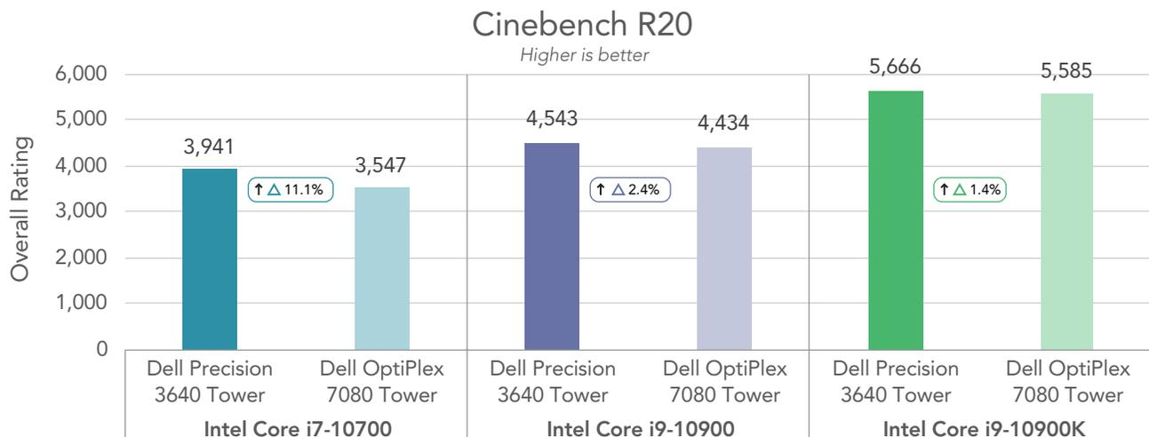
Figure 2: Cinebench R20 Overall Rating scores for the test systems. Higher is better. Source: Principled Technologies.
