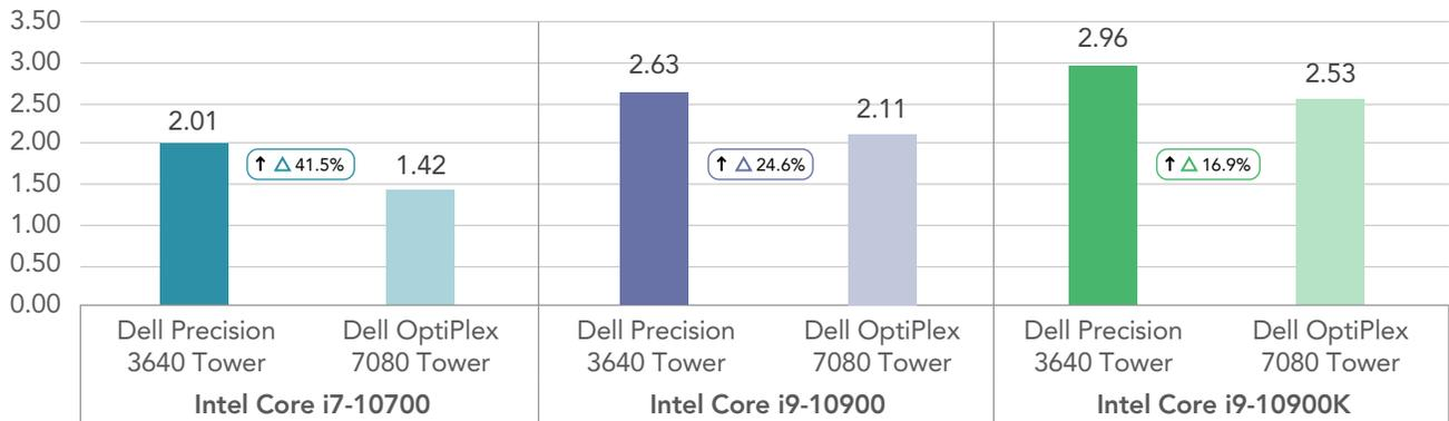
Figure 3: SPECworkstation 3 Product Development workload scores for the test systems. Higher is better. Source: Principled Technologies.
