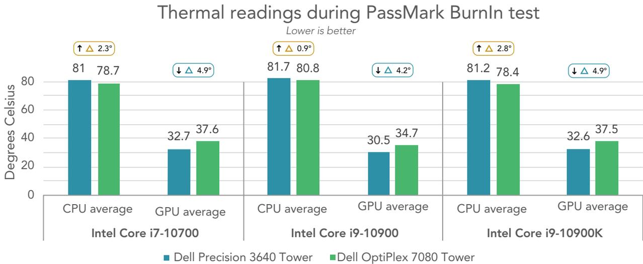
Figure 5: Thermal readings during PassMark test in degrees Celsius. Lower is better. Source: Principled Technologies.
