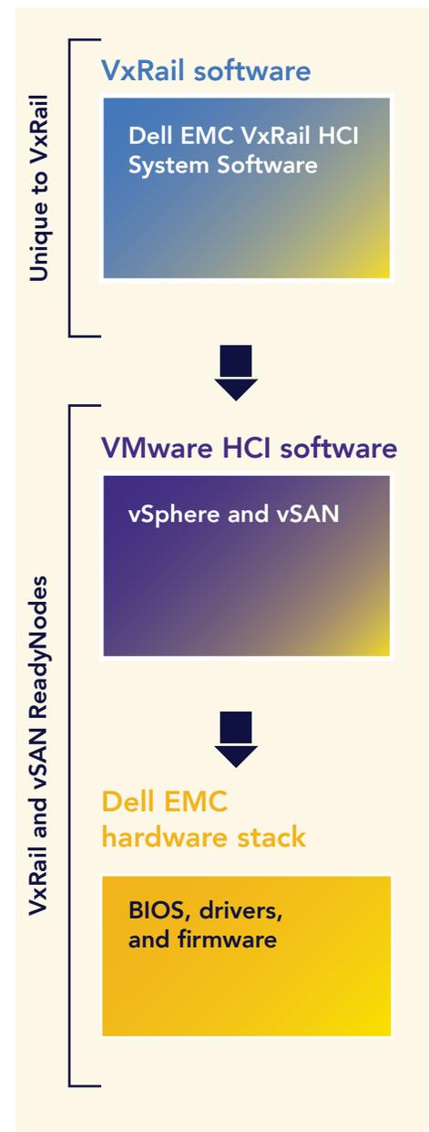
Figure 1: VxRail stack diagram.
