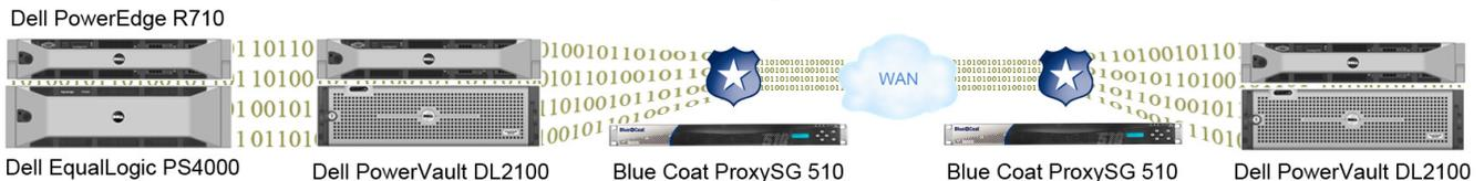
Figure 1: The high change rate scenario we tested. We used a 5Mbps effective WAN bandwidth with a 40ms round-trip latency.
