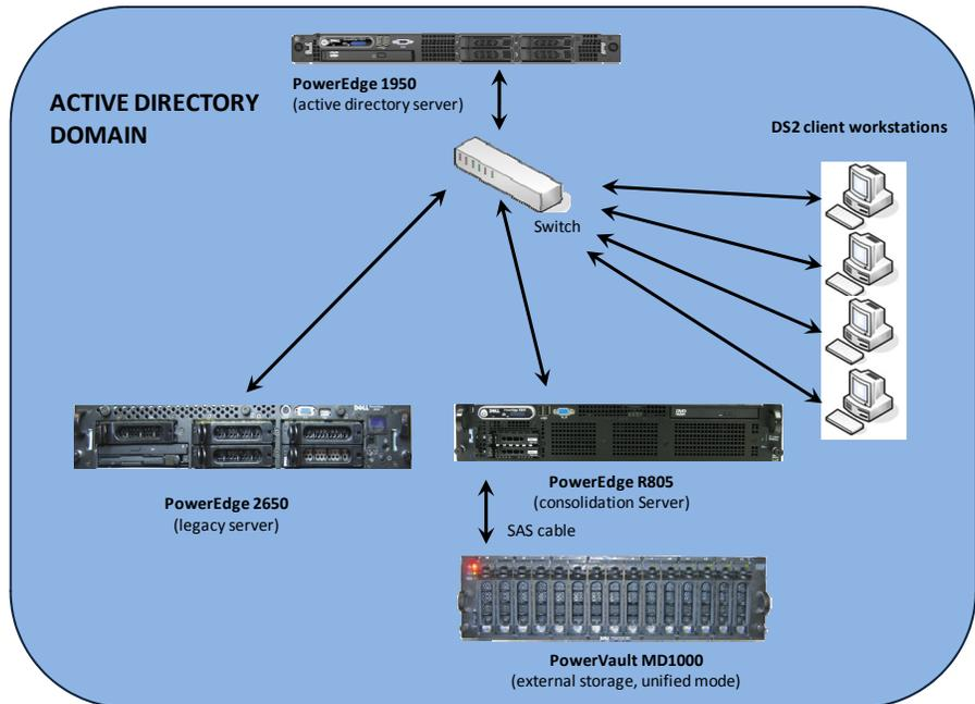
**Figure 6. The setup we used in our hands-on testing and research.**
