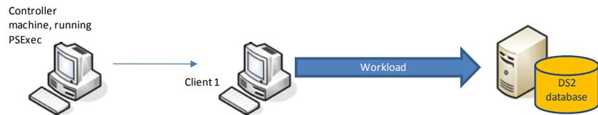
**Figure 11. Test topology for the Dell PowerEdge 2650.**
