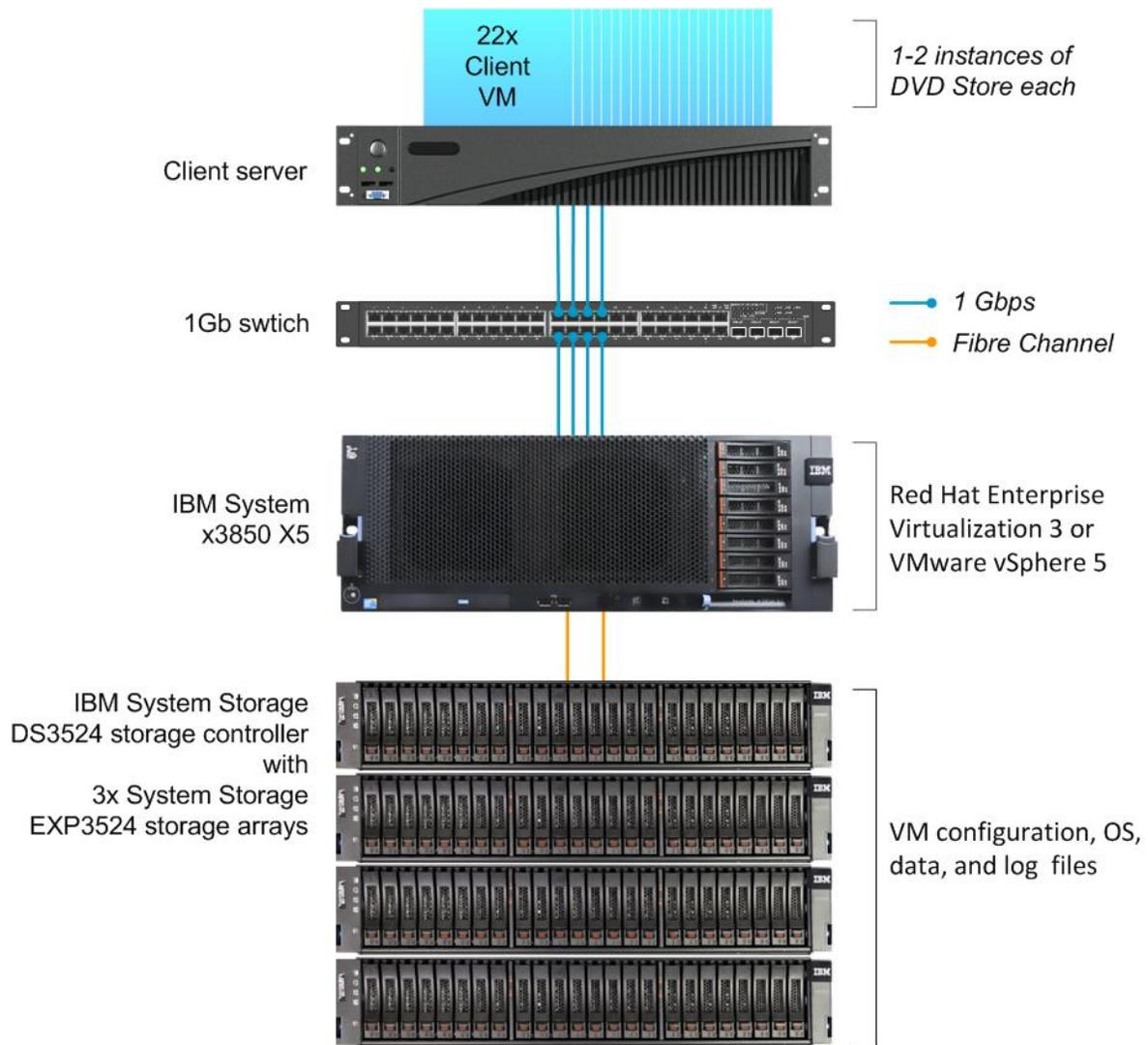
Figure 4. The test bed layout we used for both the VMware vSphere 5 and Red Hat Enterprise Virtualization 3 testing.
