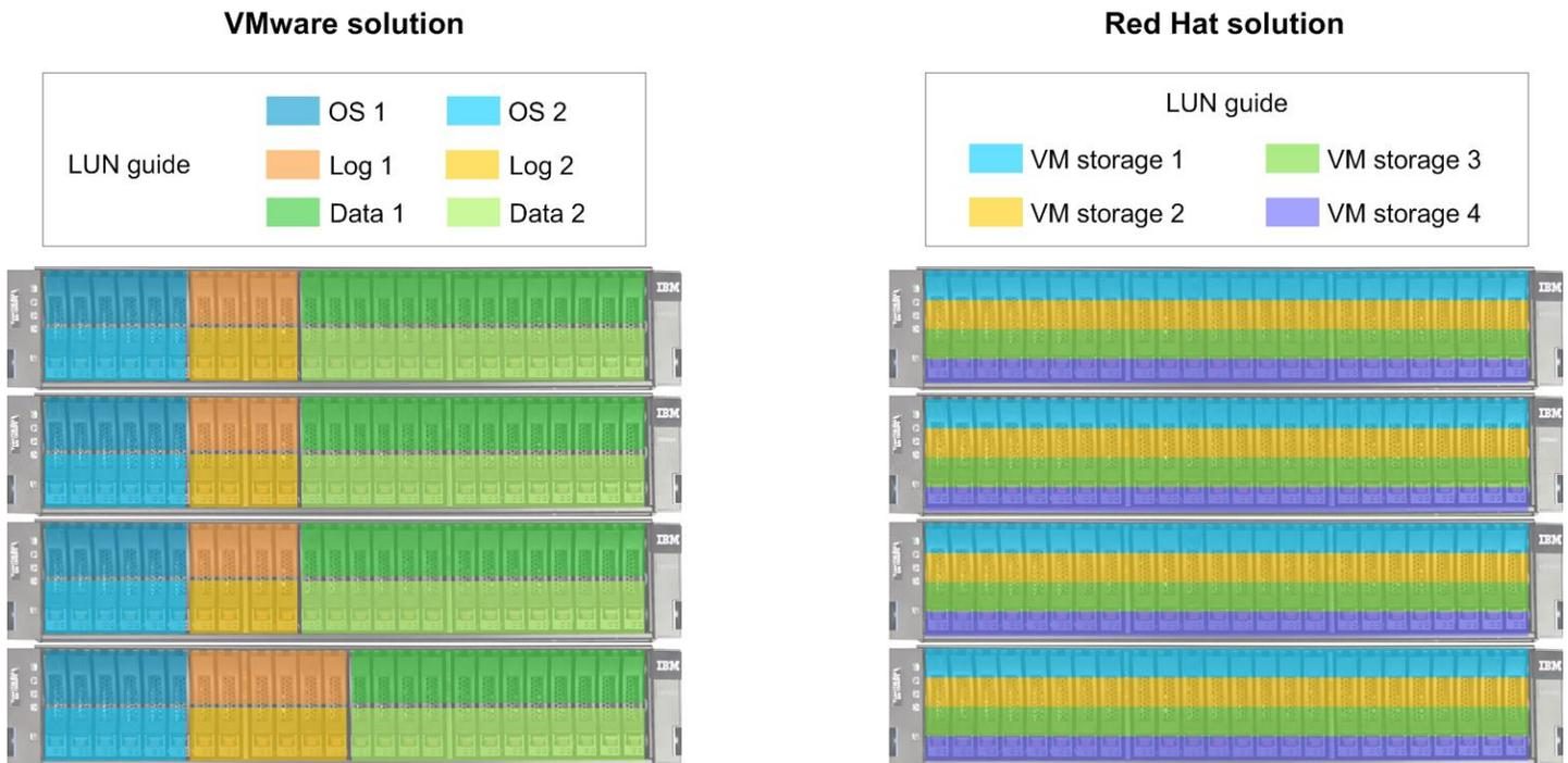
Figure 5. The storage layout we used for both the VMware vSphere 5 and Red Hat Enterprise Virtualization 3 testing.
