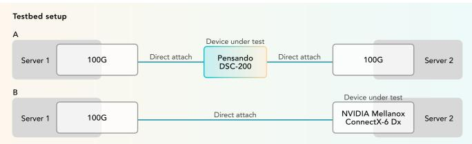
Figure 3: Our testbed setup included two HPE ProLiant DL380 servers with AMD EPYC<sup>™</sup> 7320 processors, 256 GB of memory and 16 PCIe<sup>®</sup> Gen4 risers. Source: Principled Technologies.
