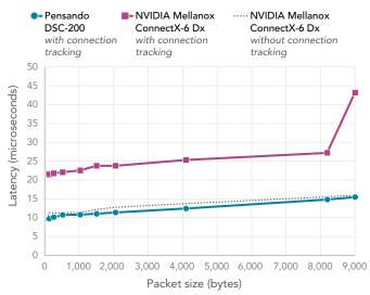
Figure 8: SDN pipeline one-way latency for the two test environments with a single instance. Lower is better. Source: Principled Technologies.
