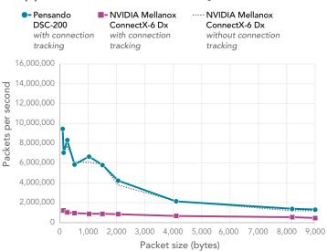
Figure 5: SDN pipeline packet rate for the two test environments with 4 instances. Higher is better. Source: Principled Technologies.
