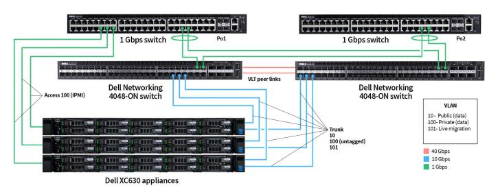
Figure 3: The network configuration for the Nutanix cluster we tested on Dell XC630 appliances.
