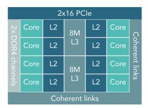
On an EPYC 7000-series processor, four Zeppelin dies connect to each other with AMD Infinity Fabric (IF) interconnect to form the AMD EPYC processor. As we show below, one EPYC processor comprises eight CCXes, 32 cores, and 64 threads.
