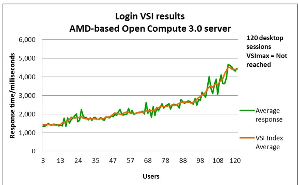
Figure 1: The AMD-based Open Compute 3.0 server supported 120 VMware Horizon View 5.2 virtual desktops.
