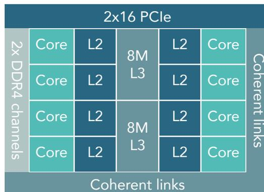
On a 7000-series processor, four Zeppelin dies connect to each other with AMD Infinity Fabric (IF) interconnect to form the AMD EPYC processor. As we show below, one EPYC processor comprises eight CcXes, 32 cores, and 64 threads.
