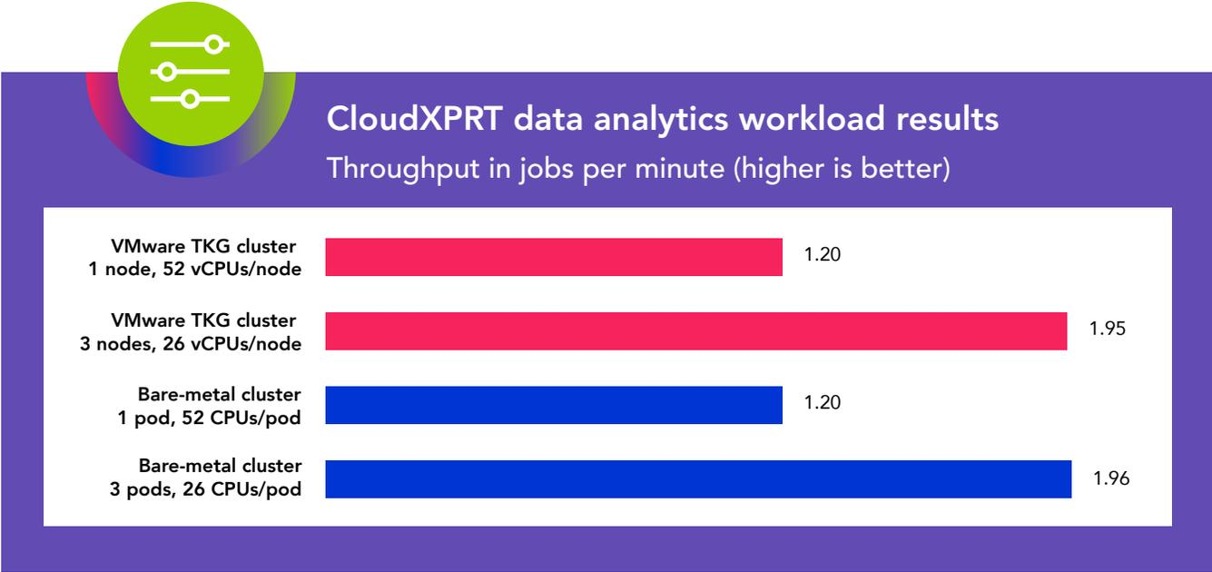
Figure 1: CloudXPRT data analytics workload throughput results for the two clusters. Higher is better. Source: Principled Technologies.
