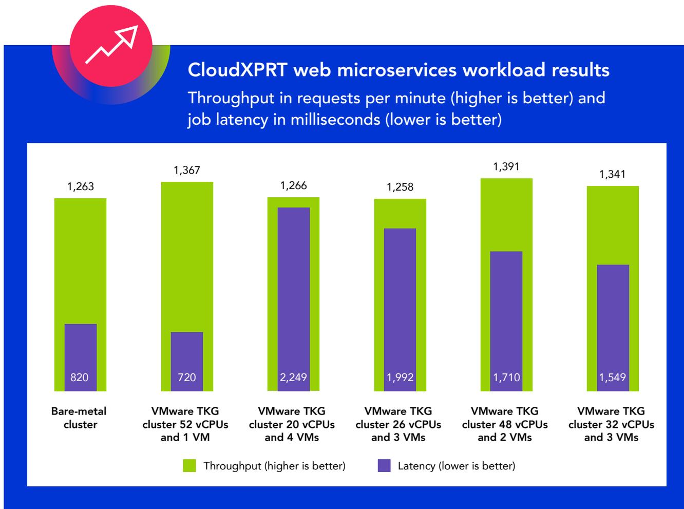
Figure 2: CloudXPRT web microservices workload results for the two clusters. Higher throughput rates and lower latencies are better. Source: Principled Technologies.
