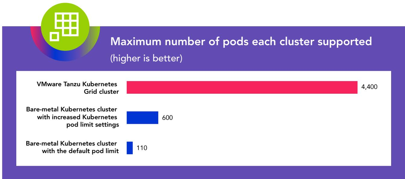
Figure 3: Maximum number of pods the two clusters supported while running a minimal web-service workload. Higher numbers are better. Source: Principled Technologies.
