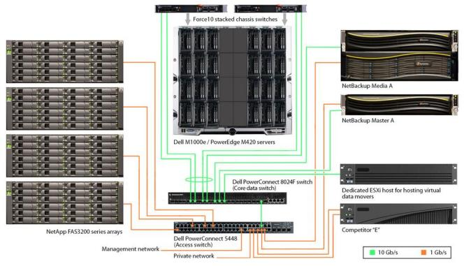
Figure 13: Detailed test bed layout: data network.
