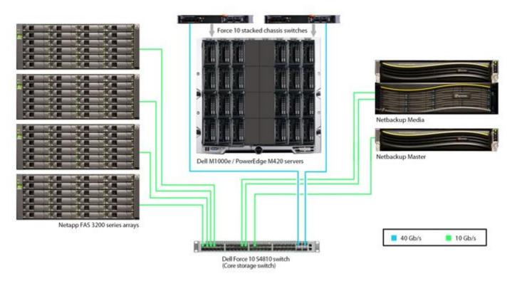
Figure 3: Detailed storage network: Storage-array snapshot-based backups.
