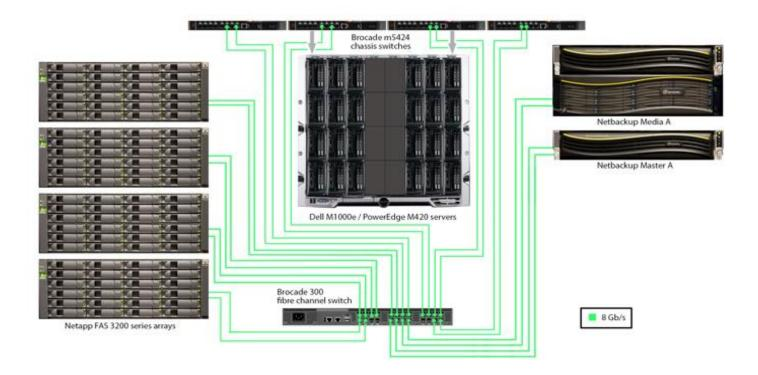
Figure 2: Detailed storage network: vStorage APIs-based backups.
