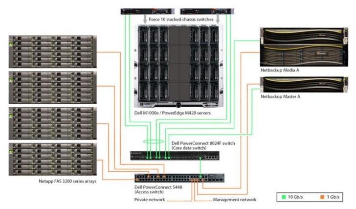
Figure 1: Detailed test bed layout: data network.
