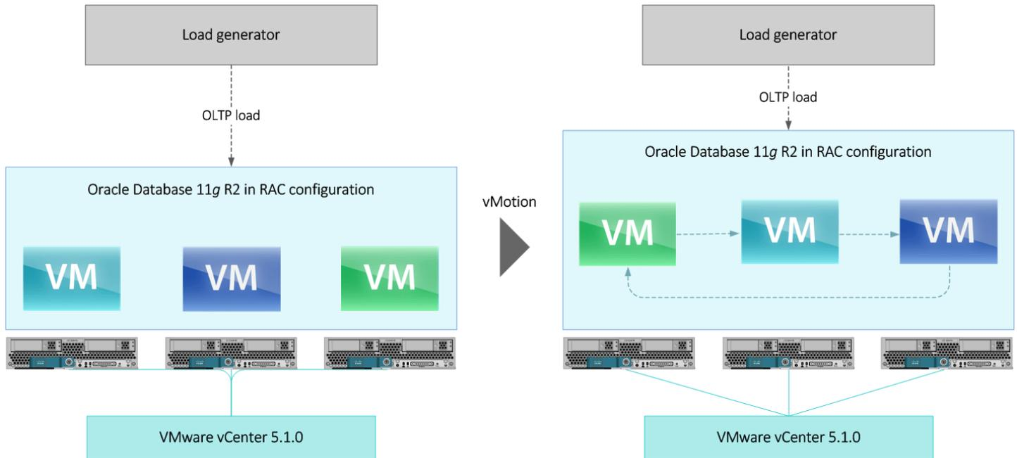
Figure 3: Diagram of our triple vMotion test, where we migrated VMs in a round-robin formation across the three hosts.
