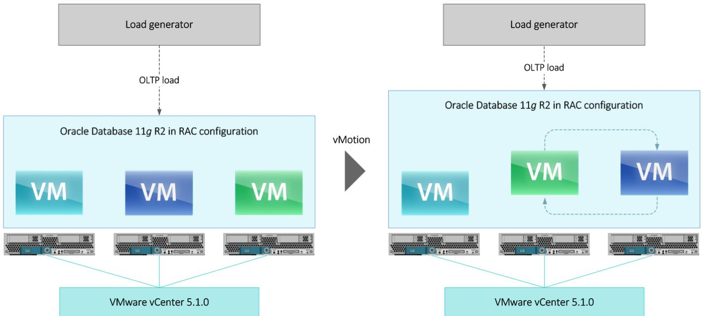
**Figure 2: Diagram of our double vMotion test, where we swapped VMs on hosts A and B.**
