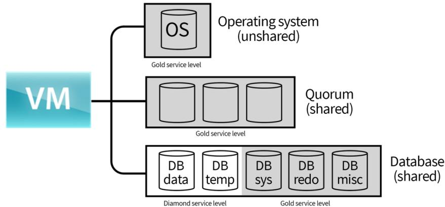
Figure 9: Logical layout of Oracle storage on the EMC VMAX Cloud Edition.
