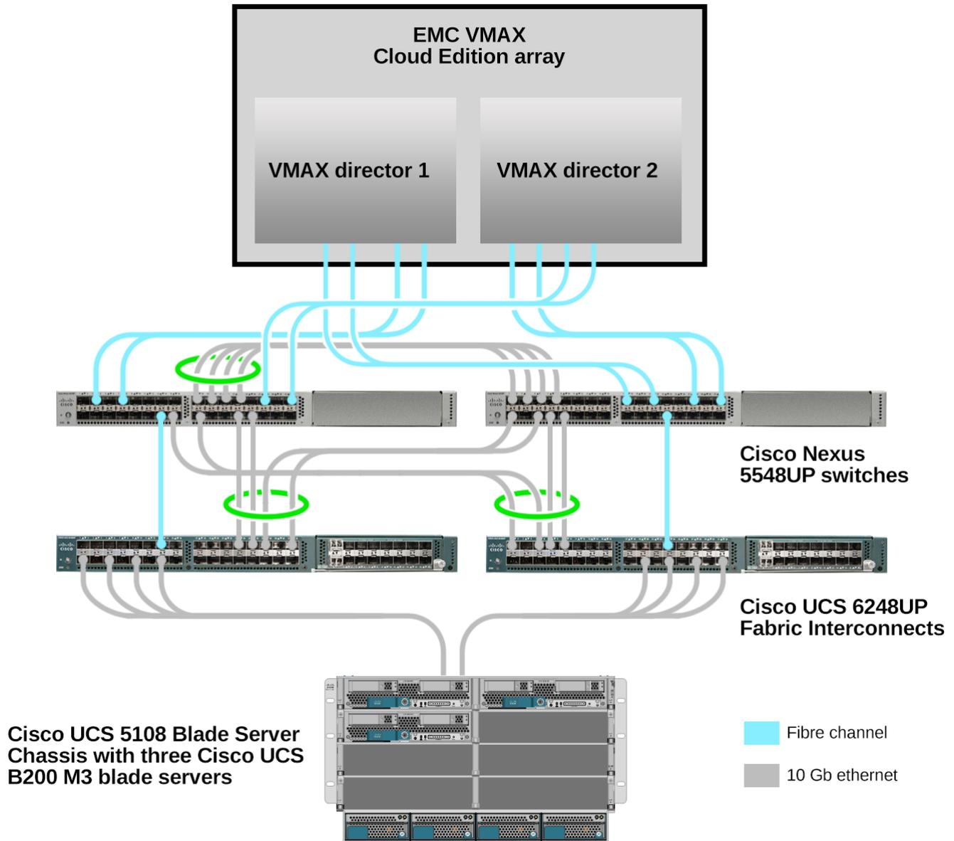
Figure 10: Diagram of the Cisco components in our test bed.
