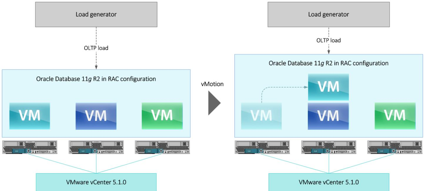
**Figure 1: Diagram of our single vMotion test, where we migrated the VM from host A to host B.**
