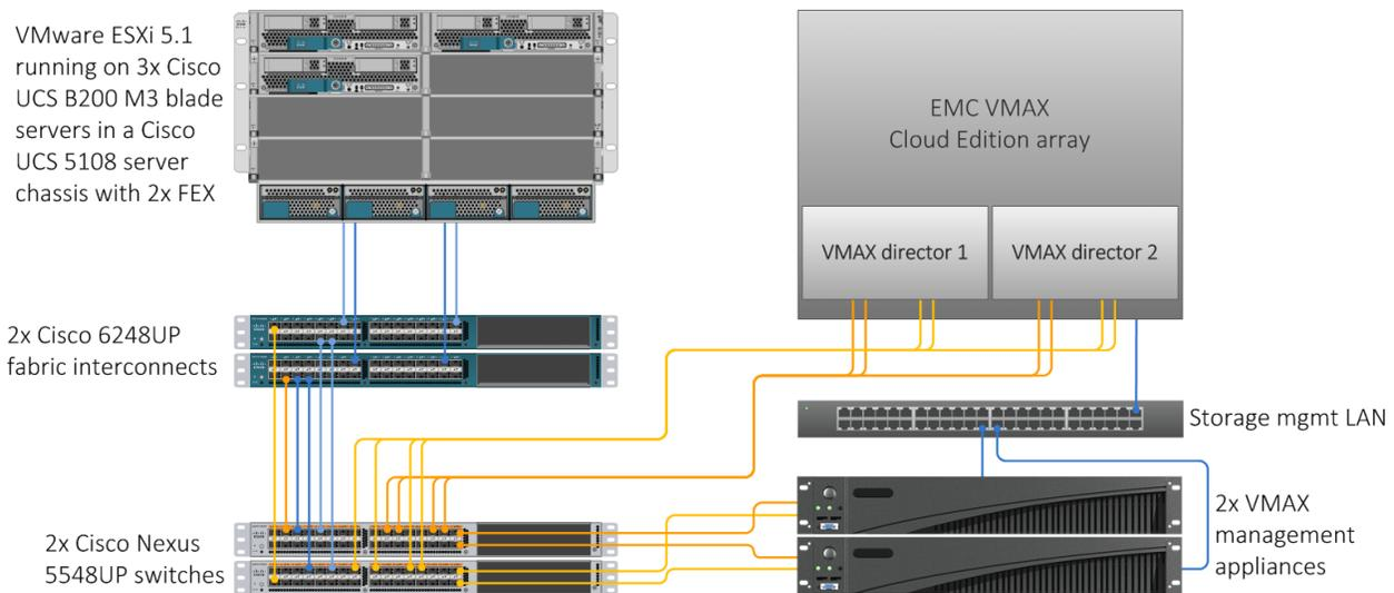
Figure 12: A diagram of our complete testbed.
