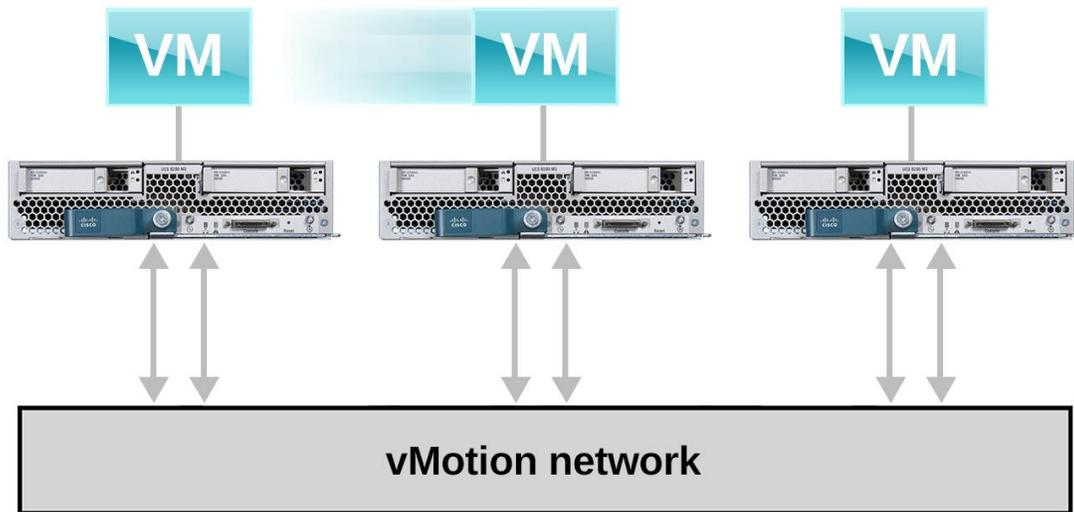
Figure 7: Each server in our test bed had two physical NICs assigned for the vMotion network.
