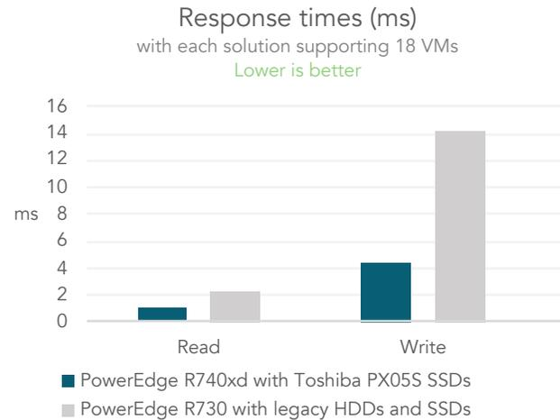
Using Toshiba PX05S SAS SSDs and VMware vSAN, Dell EMC PowerEdge R740xd servers could help businesses support customer growth and set themselves up for long-term success.
