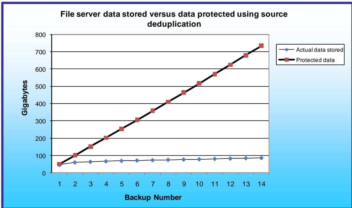
Figure 4: Comparison of protected file server data versus the actual data stored from our 2-week file server backup simulation.
