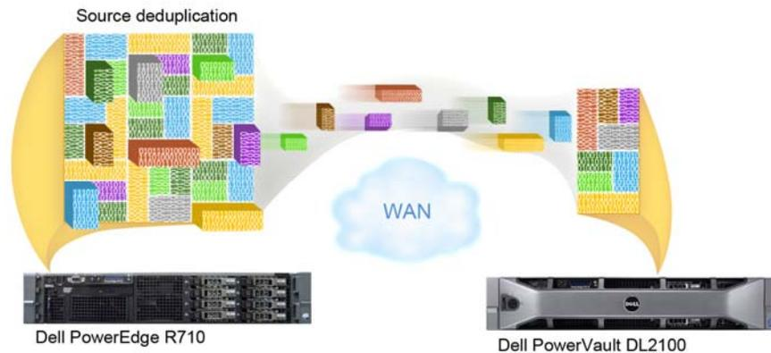
**Figure 2: Source deduplication eliminates backup inefficiencies by transferring only unique chunks of data across the WAN.**
