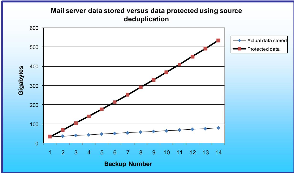
Figure 5: Comparison of protected mail server data versus the actual data stored from our 2-week Exchange 2007 backup simulation.
