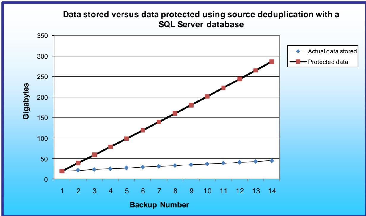
Figure 3: Comparison of protected data versus the actual data stored from our 2-week database backup simulation of a SQL Server database.
