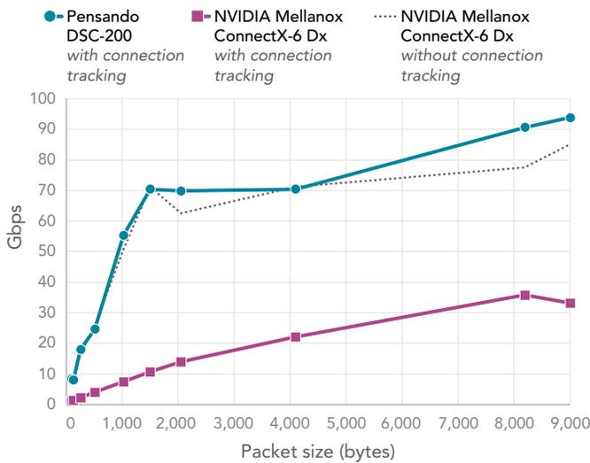
Figure 4: SDN pipeline throughput in Gbps for the two test environments with 4 instances. Higher is better. Source: Principled Technologies.
