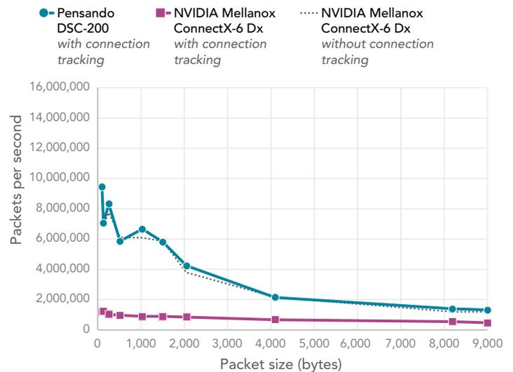
Figure 5: SDN pipeline packet rate for the two test environments with 4 instances. Higher is better. Source: Principled Technologies.
