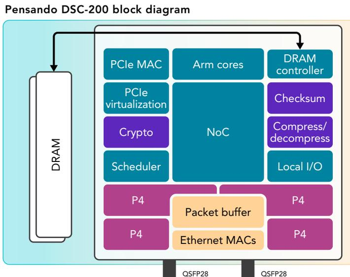
Figure 1: Pensando DSC-200 block diagram. Source: Principled Technologies, based on Figure 1 in Michael Galles and Francis Matus, "Pensando Distributed Services Architecture," IEEE Micro, 2021.<sup>3</sup>
