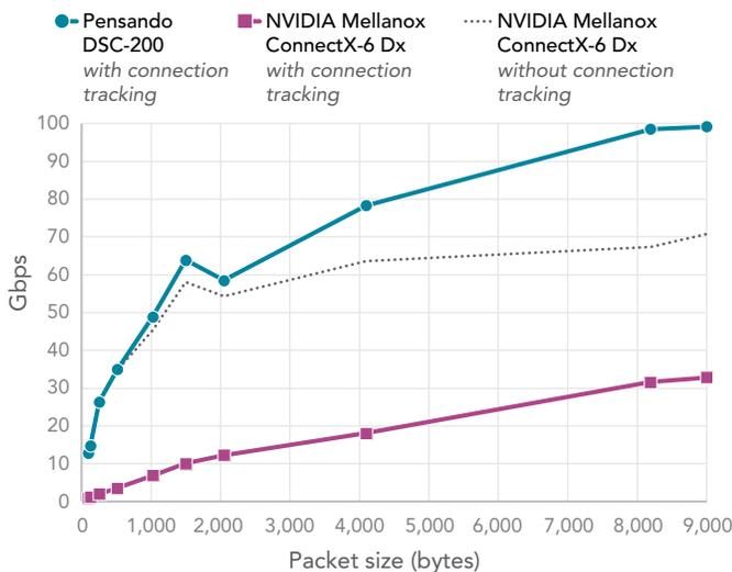
Figure 6: SDN pipeline throughput in Gbps for the two test environments with 16 instances. Higher is better. Source: Principled Technologies.
