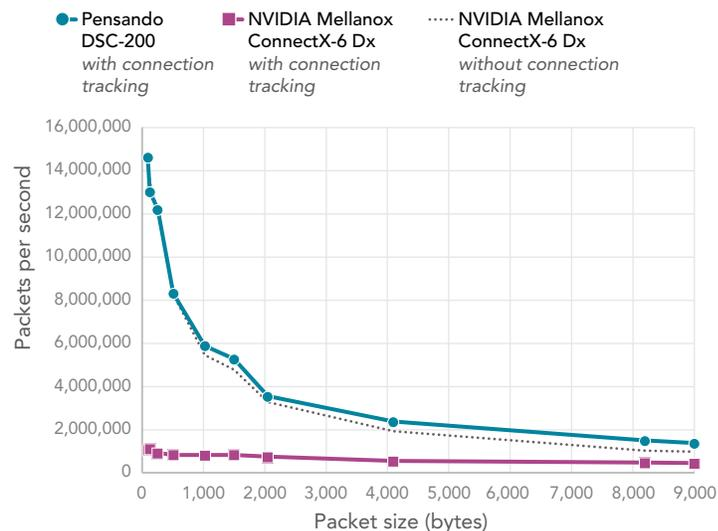
Figure 7: SDN pipeline packet rate for the two test environments with 16 instances. Higher is better. Source: Principled Technologies.
