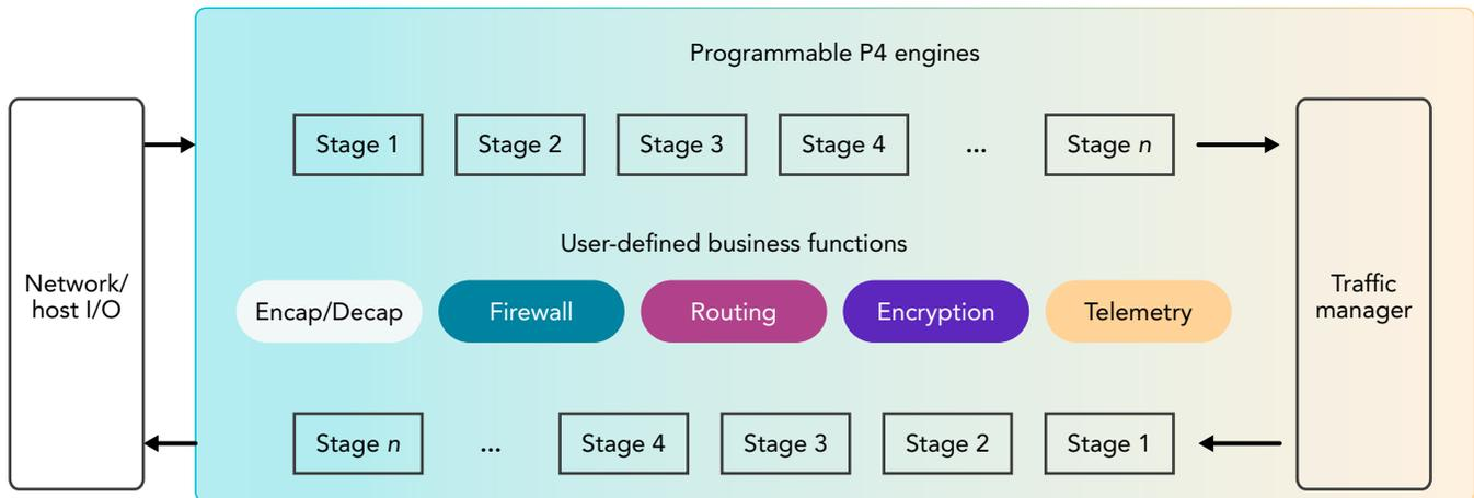
Figure 2: Programmability of the P4-programmable pipelines in the Pensando Distributed Services Card. Source: Principled Technologies, based on "Solution Brief: Distributed Services for Cloud Providers."<sup>5</sup>
