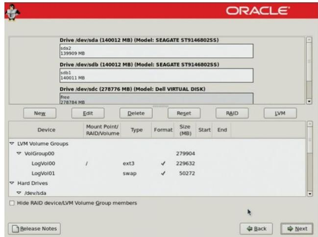
Figure 2. Remove partition and create default layout.
