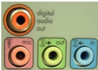
**Figure 3: The rear digital and analog audio interfaces for the AMD-based HP a1100e.**
