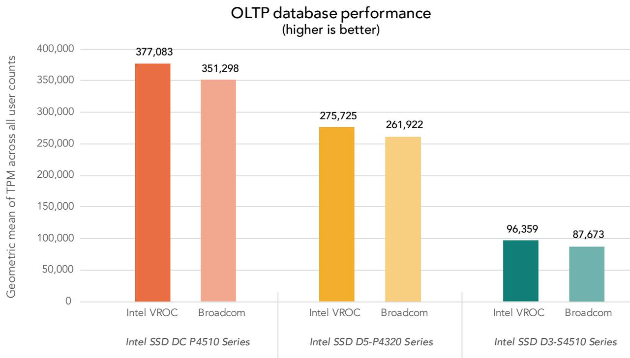
Drive choice also affects performance, particularly with workloads requiring high read I/O capabilities, like when many users require access to large databases. Using NVMe drives allows Intel VROC technology to deliver
