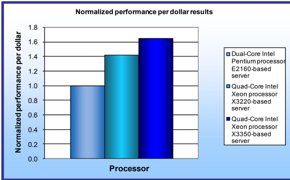
**Figure 2: Normalized performance per dollar result of the test servers across the three benchmarks. Higher numbers are better.**
