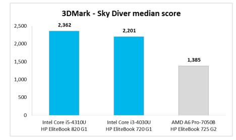
Figure 5: 3DMark Sky Diver median scores for the three test systems. Higher numbers are better.
