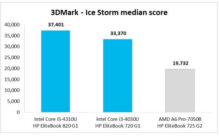
Figure 4: 3DMark Ice Storm median scores for the three test systems. Higher numbers are better.
