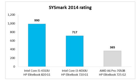
Figure 2: SYSmark 2014 scores for the three test systems. Higher scores are better.
