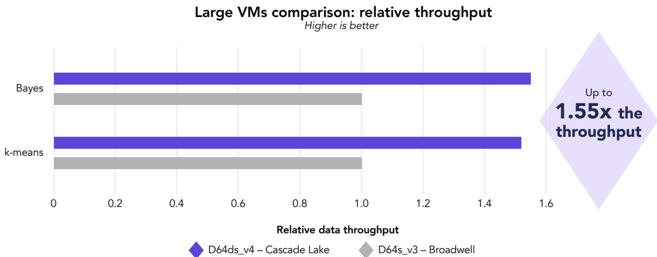
Figure 4: Normalized comparison of the average data throughput each large VM cluster achieved in the Naive Bayesian classification and k-means clustering workloads. Higher throughput is better. Source: Principled Technologies.
