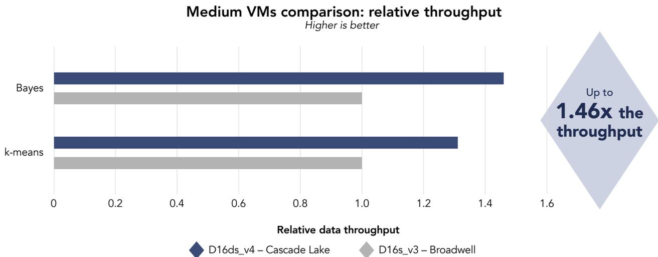
Figure 3: Normalized comparison of the average data throughput each medium VM cluster achieved in the Naïve Bayesian classification and k-means clustering workloads. Higher throughput is better. Source: Principled Technologies.
