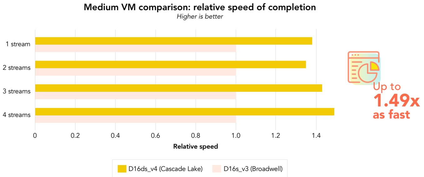
Figure 2: Comparison of the relative speed at which the medium VMs completed one, two, three, and four query streams from the TPC-H-like HammerDB workload. Greater speed is better. Source: Principled Technologies.
