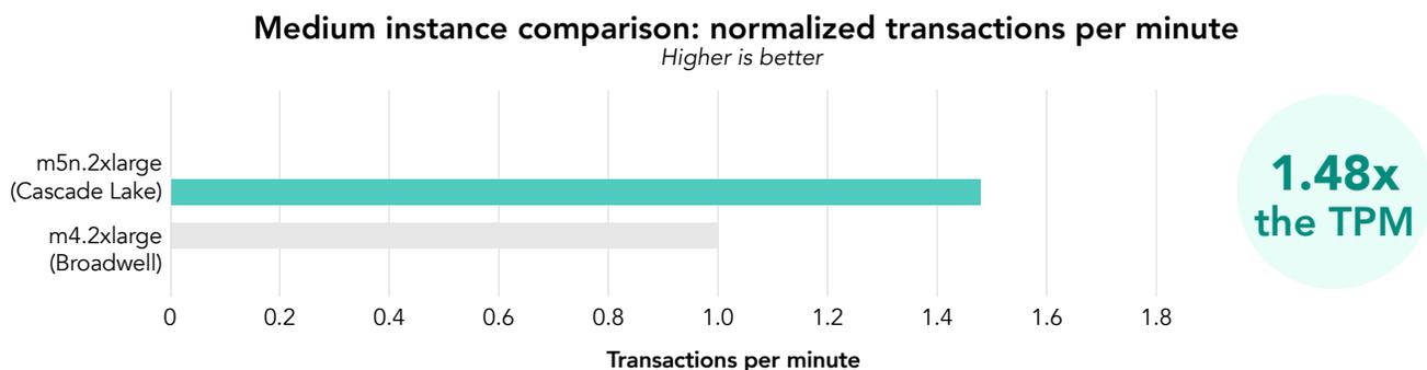
Figure 3: Normalized comparison of the average number of TPC-C-like transactions per minute each medium MySQL database instance achieved during the HammerDB workload. A higher rate is better. Source: Principled Technologies.
