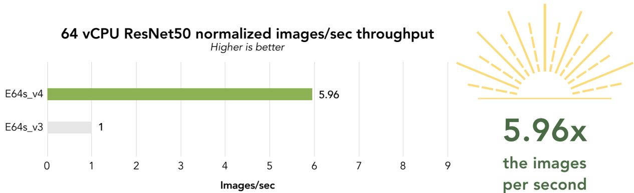
Figure 4: Relative number of images per second that the large-size VMs (64 vCPUs) classified using the ResNet50 benchmark. Higher numbers are better. Source: Principled Technologies.
