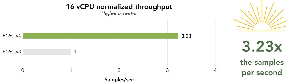
Figure 6: Relative number of samples per second that the medium-size VMs (16 vCPUs) handled using the Wide & Deep benchmark. Higher numbers are better. Source: Principled Technologies.
