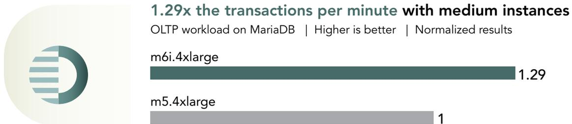
Figure 3: Comparison of average transactions per minute achieved by each 16vCPU instance, normalized to the rate achieved by the m5.4xlarge instance. Source: Principled Technologies.
