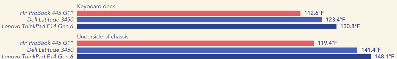
Figure 12: Median thermal results while the PCs were plugged in and running the Cinebench 2024 benchmark for 30 minutes. Lower temperatures are better. Source: Principled Technologies.
