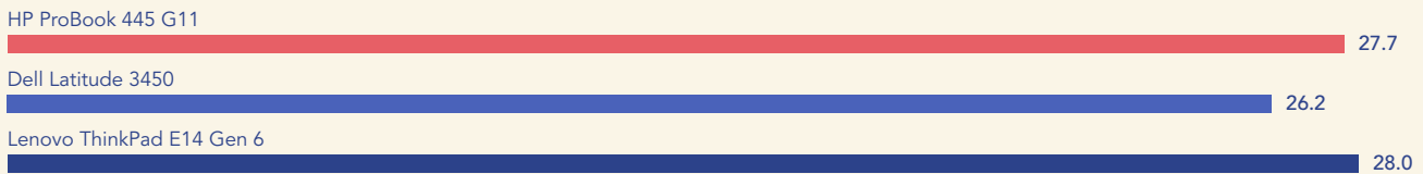
Figure 11: Median acoustic results while the PCs were plugged in and running the Cinebench 2024 benchmark for 30 minutes. Lower decibels are better. Source: Principled Technologies.
