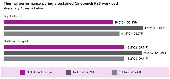
Figure 16: Temperatures under CPU load, in degrees Celsius, at two hot spots on the devices we tested. Lower numbers are better. Source: Principled Technologies.
