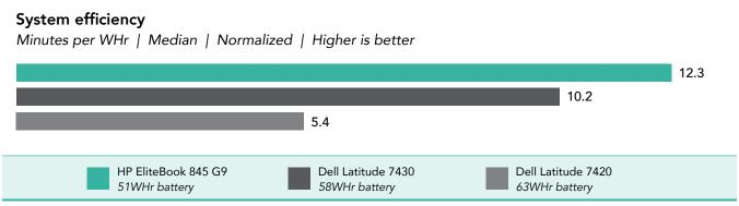
Figure 2: System efficiency of each of the three devices we tested, in minutes of battery life (as measured by the MobileMark 25 benchmark) per WHr. Higher is better. Source: Principled Technologies.
