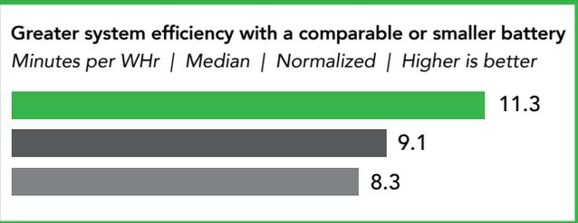
Figure 1: System efficiency of the devices we tested, in minutes of battery life (as measured by the MobileMark 2018 benchmark) per WHr. Higher is better. Source: Principled Technologies.
