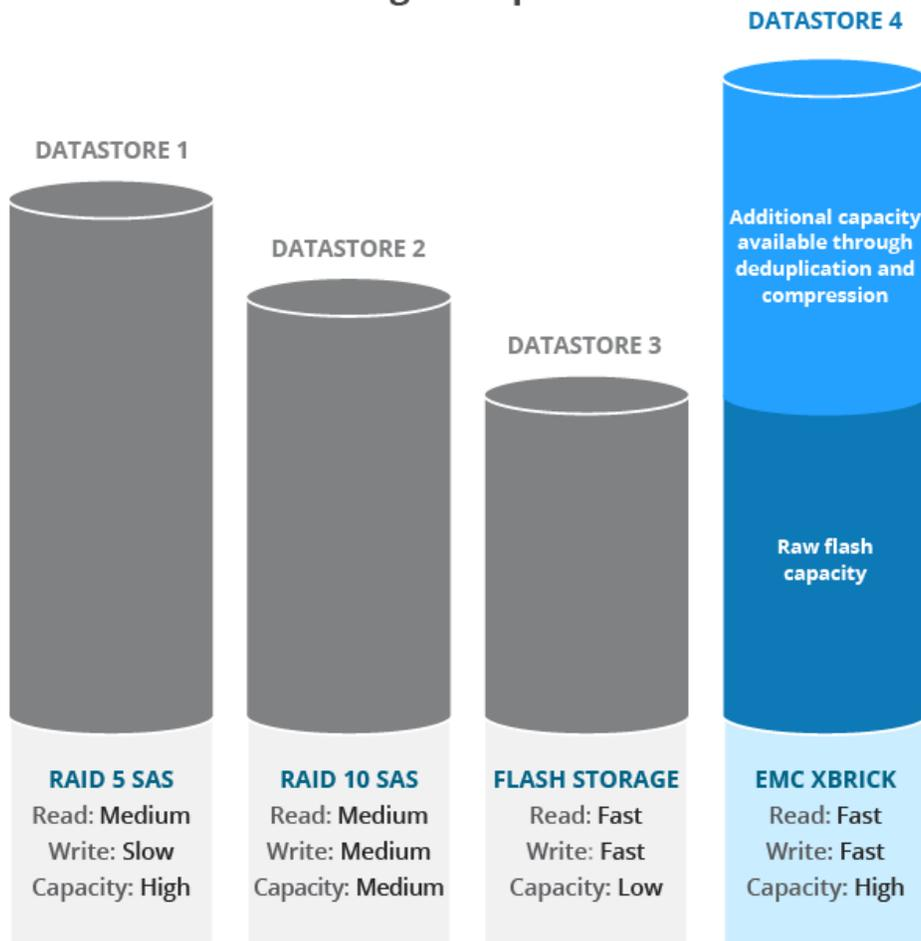
**Figure 1: The EMC X-Brick can support fast reads and writes while keeping available storage space high (addressable capacity gained by deduplication and compression will vary depending on data).**
