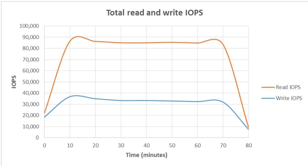
Figure 13: The total number of read and write IOPS during our median 80-minute test.
