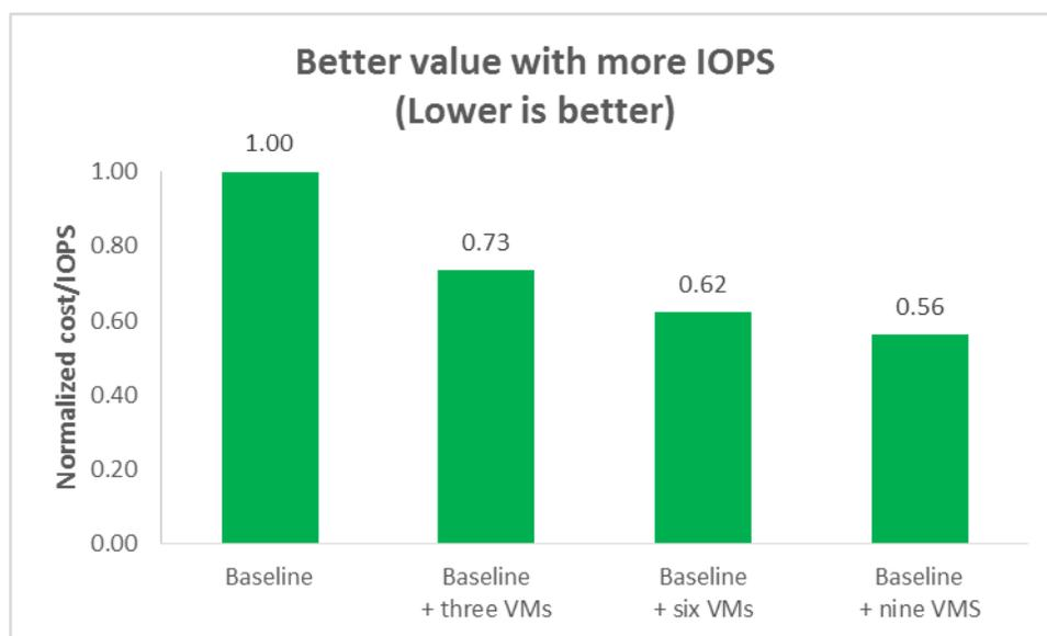
We used 1.595 TB of the array’s 30.489TB physical capacity with the max level of 13 databases. There was available capacity to add more workloads, which could then have continued to decrease the cost per logical GB and the cost per IOPS.
