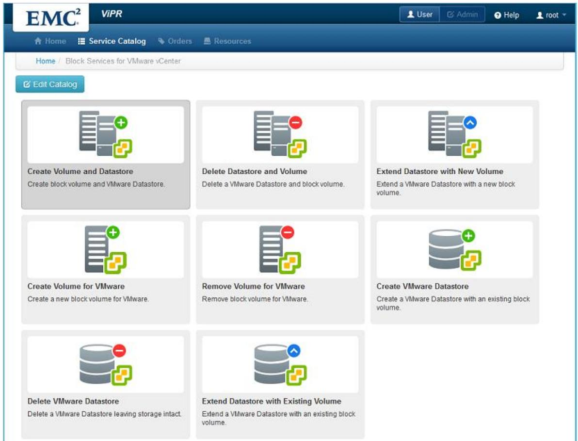
Figure 17: The service catalog provides the user self-service menu with options available to a virtualization administrator.
