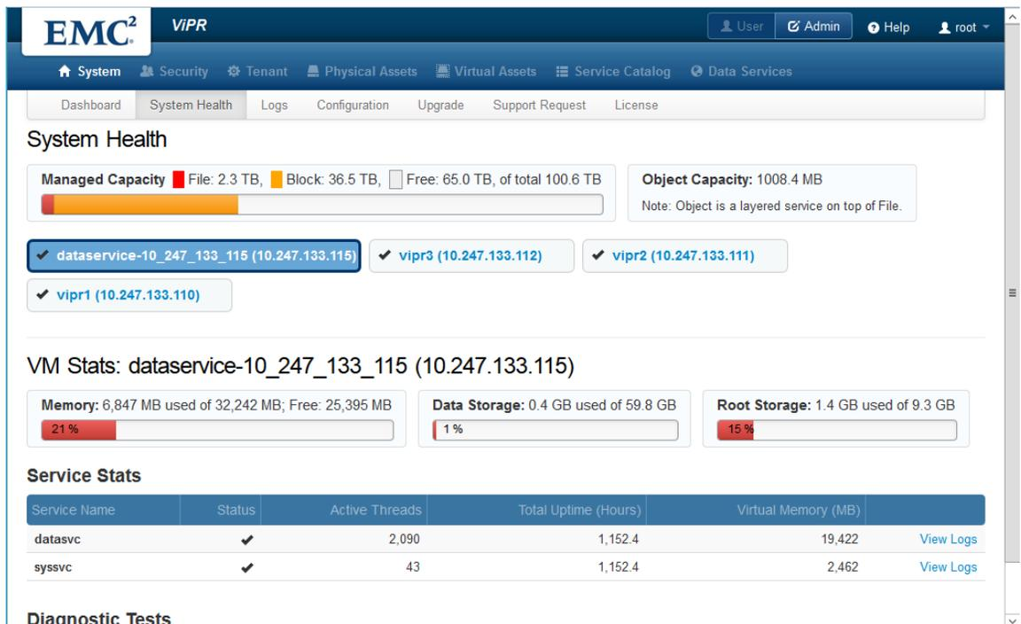
Figure 10: System Health gives a view of the statistics for each of the sub-systems within ViPR.
