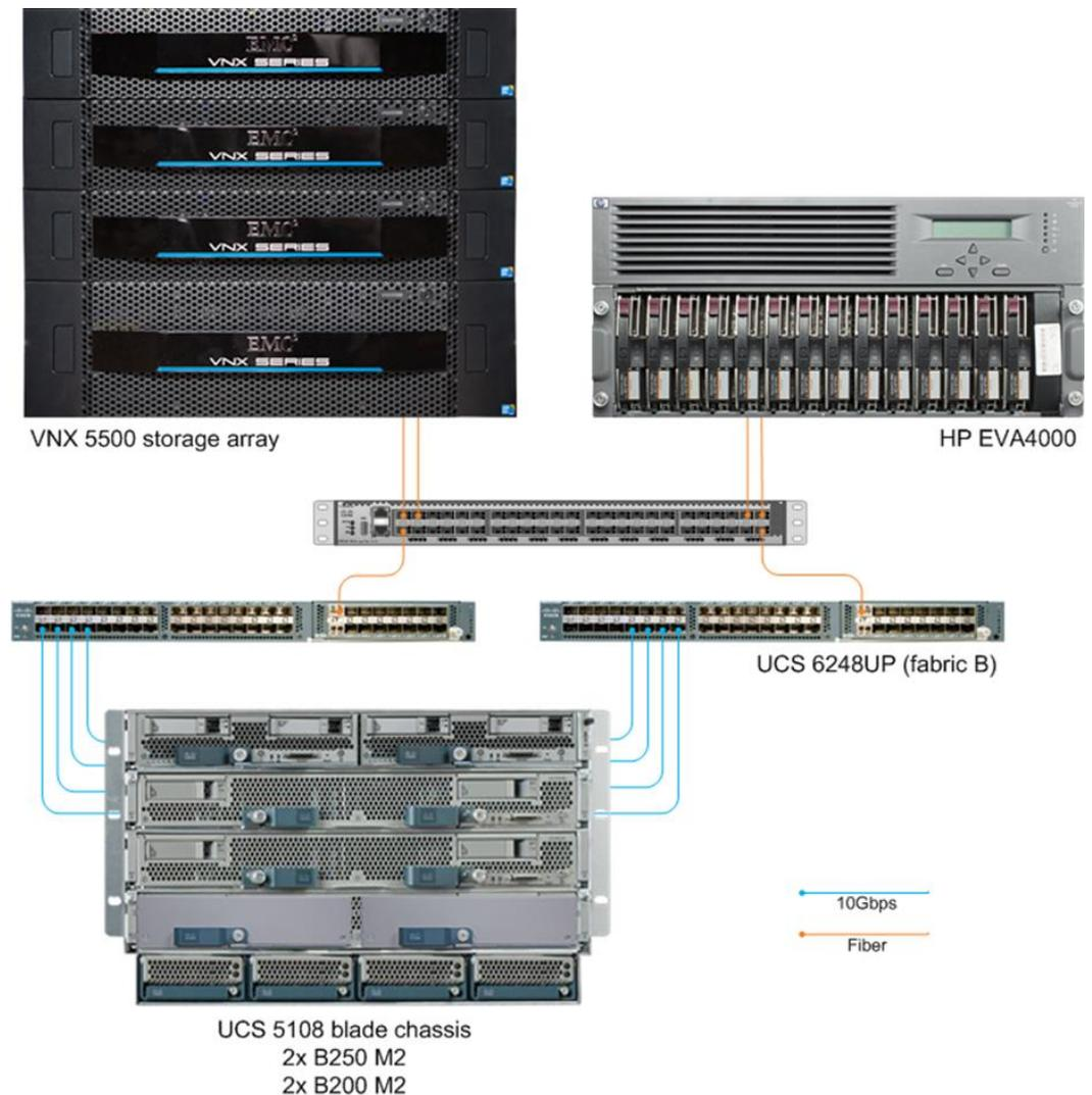
**Figure 2: Our physical lab environment with SAN connections.**
