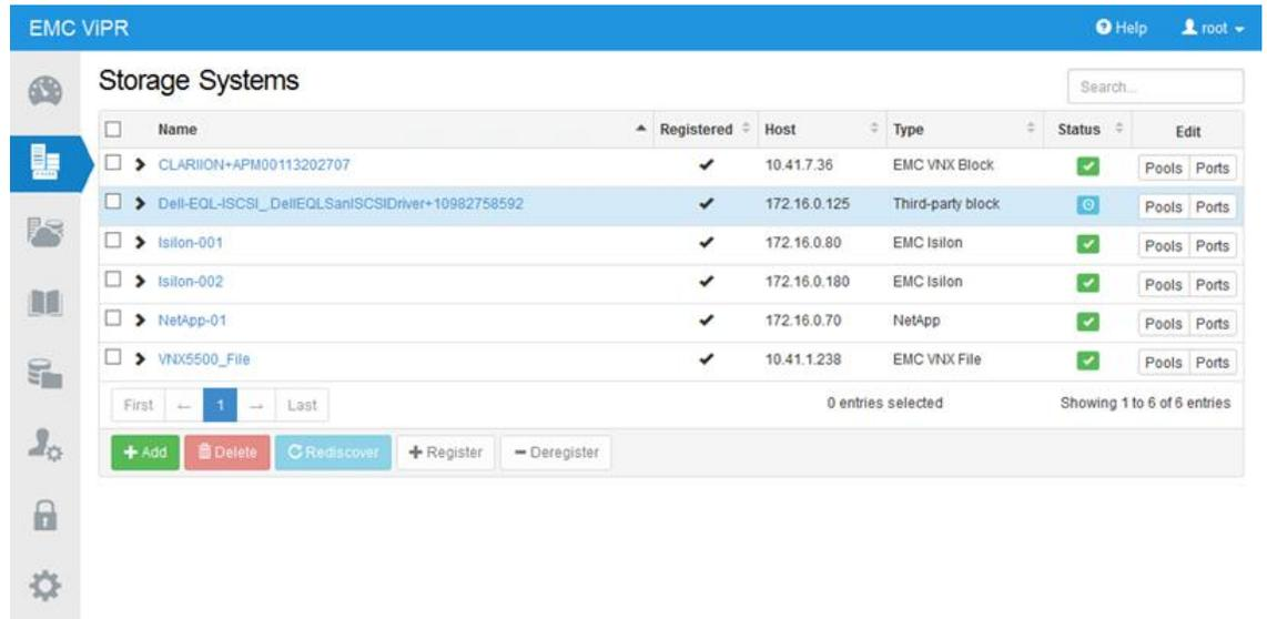
**Figure 24: ViPR Controller can integrate unsupported block storage devices leveraging OpenStack drivers.**
