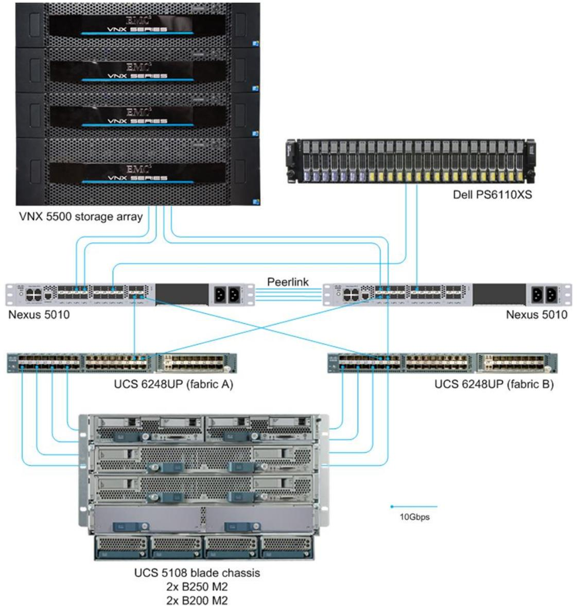
Figure 1: Our physical lab environment with data network connections.
