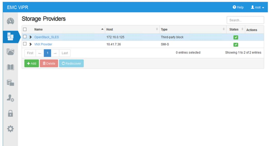
**Figure 23: EMC ViPR Controller can use OpenStack as a storage provider, enabling provisioning in otherwise unsupported storage.**
