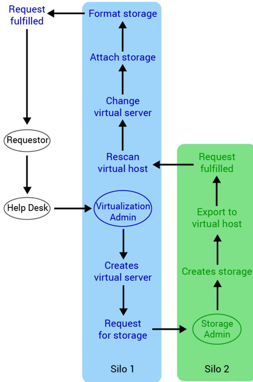
Figure 21: The manual process for provisioning a new VM with RDM disk.
