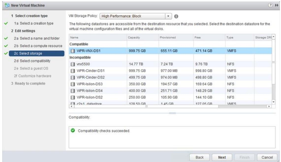
**Figure 26: The EMC ViPR Controller VASA provider gives vSphere visibility into the ViPR Controller storage pools.**
