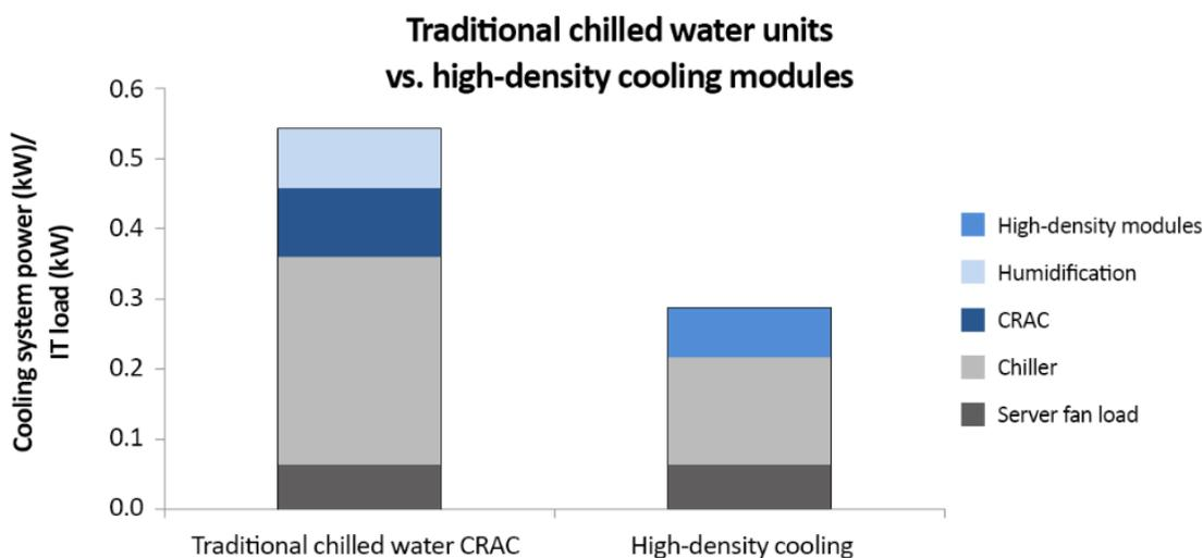
Figure 14: Traditional chilled cooling wattage versus high-density cooling module wattage.<sup>42</sup>
